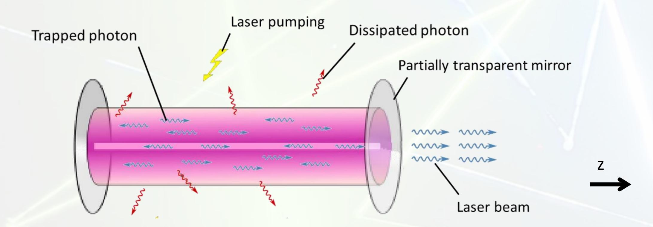
The majority of photons leave the resonator. However, photons parallel to z axis are trapped between two mirrors, which reflect them back to the gain medium. This causes an avalanche effect of stimulated emission which leads to the formation of a strong current of photons of the same frequency parallel to the z axis. Thanks to the partially transparent mirror, part of the photons leaves the resonator and forms a laser beam.
